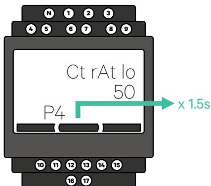
4. **FOR SOLAR CHARGING ONLY:** Access the "MEASURE" menu. Hold down the middle button for 1.5 seconds to adjust values using the left and right buttons. Change the default "A" value to "B," then press the middle button to confirm.
