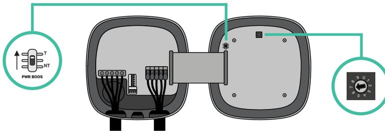
3. See the matrix below. This value must be equal or lower than the MCB protecting the Wallbox power line.
