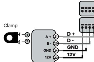
! For the N1CT installation, refer to the **Meter Configuration Guide** section.
