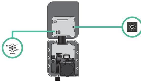
3. See the matrix below. This value must be equal or lower than the MCB protecting the Wallbox power line.
