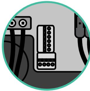
4. Once located the connector, start cabling the first charger of the chain. Check the Tools section to check if you need to use a third wire (GND).
