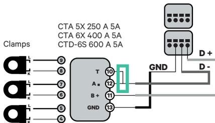
! For the EM330 configuration refer to the refer to the **Meter Configuration Guide** section.
