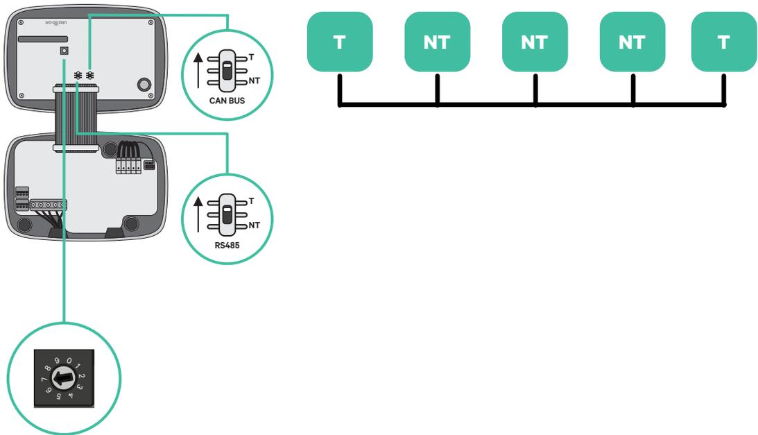
2. Once the termination resistors are set up, place the current selector of each charger following the information. The first charger of the chain is the primary charger, the others are secondary.
