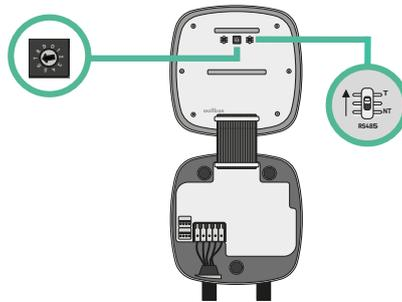
3. See the matrix below. This value must be equal or lower than the MCB protecting the Wallbox power line.
