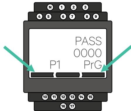
3. Using the right and left buttons, scroll up to the "Ct rAt lo" item. Press the middle button for 1.5 second and modify the value using the left and right buttons. Set it to 50 for 250 A clamp, 80 for the 400 A clamp, or 120 for the 600 A clamp. Press the middle button to confirm.
